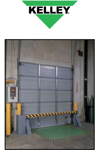
The Safety Gate can be independently operated by the dock attendant through a control panel mounted on the dock wall. The system can also be operated by a coordinated, interlocked master control panel with the operation of the dock leveler or vehicle restraint. Once the truck is restrained and the door open, the Safety Barrier opens automatically for forklift truck access. Once the door or restraint is restored the gate automatically closes.
